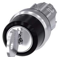
RONIS key-operated switch, 22 mm, round, metal, shiny, lock number SB30, with 2 keys, 3 switch positions I-O-II, latching, actuating angle 2x45°, 10:30h/12h/13:30h, key removal O, possible special locks: SB31, 421, 455, with laser labeling, upper case and lower case, always upper case at the beginning of the word
