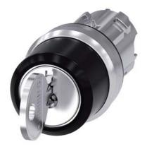
RONIS key-operated switch, 22 mm, round, metal, shiny, special lock, with 2 keys, 3 switch positions I-O-II, latching, actuating angle  $2x45^{\circ}$ , 10:30h/12h/13:30h, key removal O, possible special locks: SB31, 421, 455
