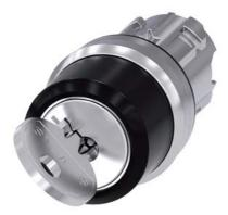
RONIS key-operated switch, 22 mm, round, metal, shiny, lock number SB30, with 2 keys, 2 switch positions O-I, latching, actuating angle 90°, 10:30h/13:30h, key removal I, possible special locks: SB31, 421, 455, Z=50-unit packaging
