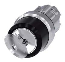
RONIS key-operated switch, 22 mm, round, metal, shiny, lock number SB30, with 2 keys, 2 switch positions O<I, momentary contact type, Actuating angle 45°, 10:30h/12h, key removal O, possible special locks: SB31, 421, 455, with laser labeling, inscription or symbol Customer-specific selection with SIRIUS ACT configurator (CIN)
