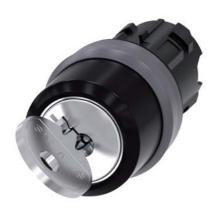
RONIS key-operated switch, 22 mm, round, plastic with metal front ring, lock number SB30, with 2 keys, 2 switch positions O<I, momentary contact type, Actuating angle 45°, 10:30h/12h, key removal O, possible special locks: SB31, 421, 455 Z=50-unit packaging
