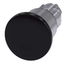
Mushroom pushbutton, 22 mm, round, metal, shiny, black, 40 mm, 3 switch positions, latches after pushing in, unlatches by pull-to-unlatch mechanism to center position, after pulling out the button Retraction to center position, with laser labeling, symbol number according to, ISO 7000 or IEC 60417
