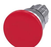
Mushroom pushbutton, 22 mm, round, metal, shiny, red, 40 mm, momentary contact type, with laser labeling, symbol number according to, ISO 7000 or IEC 60417
