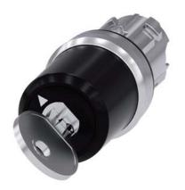
key-operated switch Siemens, 22 mm, round, metal, shiny, lock no. STGH10, with 2 keys, 2 switch positions O<I, momentary contact type, actuating angle  $45^\circ,$  10:30h/12h, key removal O, Z=50-unit packaging
