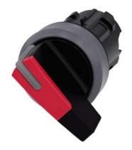
Selector switch, illuminable, 22 mm, round, plastic with metal front ring, red, selector switch, long, 2 switch positions O-I, latching, actuating angle  $90^\circ,\,10:\!30h/13:\!30h,$  with laser labeling, upper case
