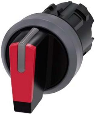
Selector switch, illuminable, 22 mm, round, plastic with metal front ring, red, selector switch, short, 3 switch positions I>O<II, momentary contact on the left, latching on the right, actuating angle 2x45°, 10:30h/12h/13:30h, with laser labeling, upper case
