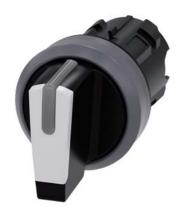
Selector switch, illuminable, 22 mm, round, plastic with metal front ring, white, selector switch, short, 3 switch positions I-O<II, left latching, right momentary contact type, actuating angle  $2x45^\circ$ , 10:30h/12h/13:30h, Z=50-unit packaging
