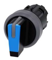
Selector switch, illuminable, 22 mm, round, plastic with metal front ring, blue, selector switch, short, 3 switch positions I-O<II, left latching, right momentary contact type, actuating angle 2x45°, 10:30h/12h/13:30h, with laser labeling, upper case
