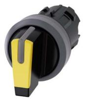
Selector switch, illuminable, 22 mm, round, plastic with metal front ring, yellow, selector switch, short, 3 switch positions I-O<II, left latching, right momentary contact type, actuating angle 2x45°, 10:30h/12h/13:30h, with laser labeling, inscription or symbol Customer-specific selection with SIRIUS ACT configurator (CIN)
