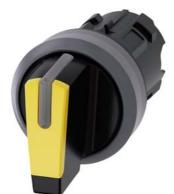
Selector switch, illuminable, 22 mm, round, plastic with metal front ring, yellow, selector switch, short, 3 switch positions I-O<II, left latching, right momentary contact type, actuating angle  $2x45^{\circ}$ , 10:30h/12h/13:30h, with laser labeling, lower case
