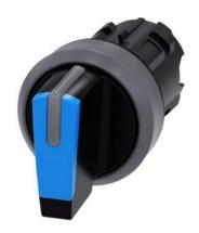
Selector switch, illuminable, 22 mm, round, plastic with metal front ring, blue, selector switch, short, 3 switch positions I>O<II, momentary contact type, actuating angle  $2x45^{\circ}$ , 10:30h/12h/13:30h, with laser labeling, lower case
