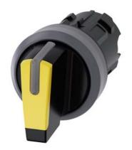
Selector switch, illuminable, 22 mm, round, plastic with metal front ring, yellow, selector switch, short, 3 switch positions I>O<II, momentary contact type, actuating angle  $2x45^{\circ}$ , 10:30h/12h/13:30h, with laser labeling, lower case
