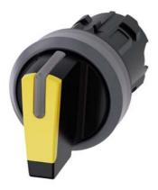
Selector switch, illuminable, 22 mm, round, plastic with metal front ring, yellow, selector switch, short, 3 switch positions I>O<II, momentary contact type, actuating angle 2x45°, 10:30h/12h/13:30h, with laser labeling, upper case and lower case, always upper case at beginning of line
