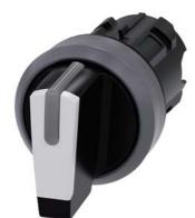
Selector switch, illuminable, 22 mm, round, plastic with metal front ring, white, selector switch, short, 3 switch positions I-O-II, latching, actuating angle 2x45°, 10:30h/12h/13:30h, with laser labeling, inscription or symbol Customer-specific selection with SIRIUS ACT configurator (CIN)
