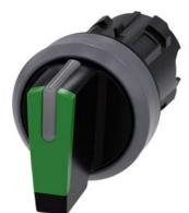
Selector switch, illuminable, 22 mm, round, plastic with metal front ring, green, selector switch, short, 3 switch positions I-O-II, latching, actuating angle 2x45°, 10:30h/12h/13:30h, with laser labeling, lower case
