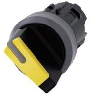
Selector switch, illuminable, 22 mm, round, plastic with metal front ring, yellow, selector switch, short, 2 switch positions O-I, latching, actuating angle  $90^\circ$ , 10:30h/13:30h, with laser labeling, lower case
