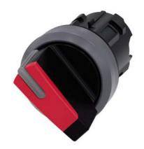
Selector switch, illuminable, 22 mm, round, plastic with metal front ring, red, selector switch, short, 2 switch positions O-I, latching, actuating angle 90°, 10:30h/13:30h, with laser labeling, upper case
