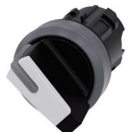
Selector switch, illuminable, 22 mm, round, plastic with metal front ring, white, selector switch, short, 2 switch positions O<I, momentary contact type, Actuating angle 45°, 10:30h/12h, with laser labeling, upper case
