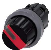
Selector switch, illuminable, 22 mm, round, plastic with metal front ring, red, Rotary knob, 2 switch positions O-I, latching, actuating angle 90°, 10:30h/13:30h, Z=50-unit packaging
