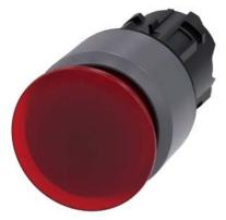
Illuminated mushroom pushbutton, 22 mm, round, plastic with metal front ring, red, 30 mm, latching, pull-to-unlatch mechanism, with laser labeling, upper case and lower case, always upper case at beginning of line
