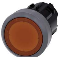
Illuminated pushbutton, 22 mm, round, plastic with metal front ring, amber, pushbutton, flat momentary contact type, with laser labeling, symbol number according to, ISO 7000 or IEC 60417
