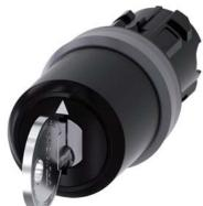
Key-operated switch IKON, 22 mm, round, plastic with metal front ring, lock number 360012K1, with 2 keys, 3 switch positions I-O-II, latching, actuating angle 2x45°, 10:30h/12h/13:30h, key removal O, with laser labeling, upper case and lower case, always upper case at the beginning of the word
