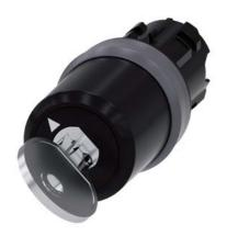
Key-operated switch BKS, 22 mm, round, plastic with metal front ring, lock No. E9 (VW), without key, 2 switch positions O-I, latching, actuating angle  $90^\circ, 10:30h/13:30h,$  key removal O+I, with laser labeling, upper case and lower case, always upper case at beginning of line
