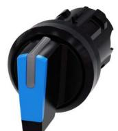
Selector switch, illuminable, 22 mm, round, plastic, blue, selector switch, short, 3 switch positions I>O<II, momentary contact on the left, latching on the right, actuating angle 2x45°, 10:30h/12h/13:30h, with laser labeling, upper case and lower case, always upper case at beginning of line
