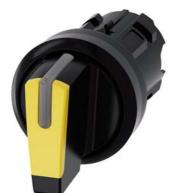
Selector switch, illuminable, 22 mm, round, plastic, yellow, selector switch, short, 3 switch positions I>O<II, momentary contact on the left, latching on the right, actuating angle 2x45°, 10:30h/12h/13:30h Z=50-unit packaging
