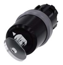
key-operated switch Siemens, 22 mm, round, plastic with metal front ring, lock no. LSG1, with 2 keys, 2 switch positions O<I, momentary contact type, actuating angle 45°, 10:30h/12h, key removal O, with laser labeling, upper case and lower case, always upper case at beginning of line
