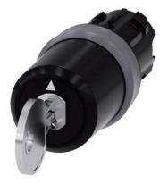
key-operated switch Siemens, 22 mm, round, plastic with metal front ring, lock number SSG10, with 2 keys, 3 switch positions I-O<II, left latching, momentary contact type on the right, actuating angle  $2x45^\circ$ , 10:30h/12h/13:30h, key removal O+I, with laser labeling, upper case and lower case, always upper case at the beginning of the word
