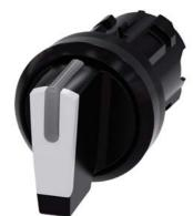
Selector switch, illuminable, 22 mm, round, plastic, white, selector switch, short, 3 switch positions I-O<II, left latching, right momentary contact type, actuating angle 2x45°, 10:30h/12h/13:30h, with laser labeling, upper case
