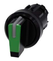
Selector switch, illuminable, 22 mm, round, plastic, green, selector switch, short, 3 switch positions I-O<II, left latching, right momentary contact type, actuating angle  $2x45^{\circ}$ , 10:30h/12h/13:30h, with laser labeling, upper case and lower case, always upper case at beginning of line
