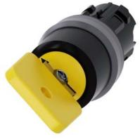
Key-operated switch O.M.R, 22 mm, round, plastic with metal front ring, lock number 73033, yellow, with 2 keys, 2 switch positions O-I, latching, actuating angle 90°, 10:30h/13:30h, key removal O+I, with laser labeling, upper case and lower case, always upper case at the beginning of the word
