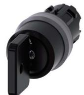
Key-operated switch O.M.R, 22 mm, round, plastic with metal front ring, lock number 73034, black, with 2 keys, 3 switch positions I>O<II, momentary contact type, actuating angle 2x45°, 10:30h/12h/13:30h, key removal O, with laser labeling, lower case
