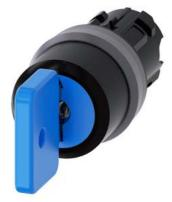
Key-operated switch O.M.R, 22 mm, round, plastic with metal front ring, lock number 73038, blue, with 2 keys, 3 switch positions I-O<II, left latching, right momentary contact type, actuating angle 2x45°, 10:30h/12h/13:30h, key removal O, with laser labeling, upper case and lower case, always upper case at the beginning of the word
