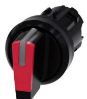
Selector switch, illuminable, 22 mm, round, plastic, red, selector switch, short, 3 switch positions >O<II, momentary contact type, actuating angle 2x45°, 10:30h/12h/13:30h, with laser labeling, inscription or symbol Customer-specific selection with SIRIUS ACT configurator (CIN)
