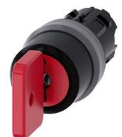
Key-operated switch O.M.R, 22 mm, round, plastic with metal front ring, lock number 73037, red, with 2 keys, 3 switch positions I-O-II, latching, actuating angle 2x45°, 10:30h/12h/13:30h, key removal O, with laser labeling, upper case and lower case, always upper case at beginning of line
