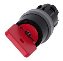
Key-operated switch O.M.R, 22 mm, round, plastic with metal front ring, lock number 73037, red, with 2 keys, 2 switch positions O-I, latching, actuating angle 90°, 10:30h/13:30h, key removal O, with laser labeling, upper case and lower case, always upper case at the beginning of the word
