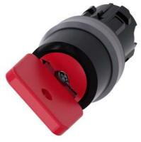
Key-operated switch O.M.R, 22 mm, round, plastic with metal front ring, lock number 73037, red, with 2 keys, 2 switch positions O-I, latching, actuating angle 90°, 10:30h/13:30h, key removal O, Z=50-unit packaging
