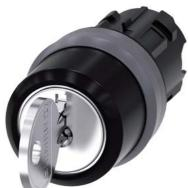
RONIS key-operated switch, 22 mm, round, plastic with metal front ring, lock number 455, with 2 keys, 3 switch positions I-O-II, latching, actuating angle 2x45°, 10:30h/12h/13:30h, Key removal I+O+II, with laser labeling, upper case and lower case, always upper case at the beginning of the word
