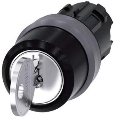
RONIS key-operated switch, 22 mm, round, plastic with metal front ring, lock number 455, with 2 keys, 3 switch positions I-O-II, latching, actuating angle 2x45°, 10:30h/12h/13:30h, Key removal I+O+II, with laser labeling, upper case
