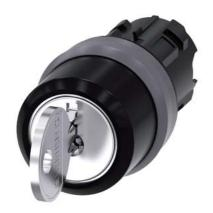
RONIS key-operated switch, 22 mm, round, plastic with metal front ring, lock number SB30, with 2 keys, 3 switch positions I>O<II, momentary contact on the left, latching on the right, actuating angle 2x45°, 10:30h/12h/13:30h, Key removal II, possible special locks: SB31, 421, 455, Z=50-unit packaging
