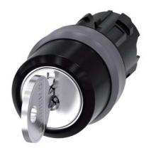
RONIS key-operated switch, 22 mm, round, plastic with metal front ring, lock number SB30, with 2 keys, 3 switch positions I>O<II, momentary contact type, actuating angle  $2x45^{\circ}$ , 10:30h/12h/13:30h, key removal O, possible special locks: SB31, 421, 455, with laser labeling, upper case
