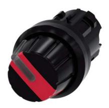
Selector switch, illuminable, 22 mm, round, plastic, red, Rotary knob, 2 switch positions O-I, latching, actuating angle 90°, 10:30h/13:30h, with laser labeling, lower case
