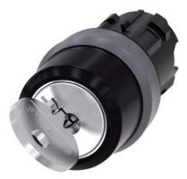
RONIS key-operated switch, 22 mm, round, plastic with metal front ring, lock number SB30, with 2 keys, 2 switch positions O-I, latching, actuating angle 90°, 10:30h/13:30h, key removal O+I, possible special locks: SB31, 421, 455, with laser labeling, inscription or symbol Customer-specific selection with SIRIUS ACT configurator (CIN)
