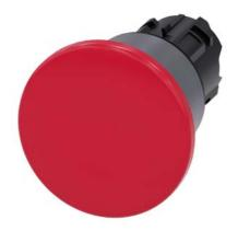
Mushroom pushbutton, 22 mm, round, plastic with metal front ring, red, 40mm, latching, pull-to-unlatch mechanism, with laser labeling, inscription or symbol Customer-specific selection with SIRIUS ACT configurator (CIN)
