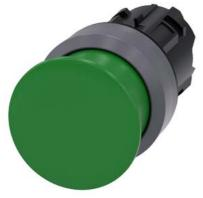
Mushroom pushbutton, 22 mm, round, plastic with metal front ring, green, 30 mm, momentary contact type, with laser labeling, upper case and lower case, always upper case at the beginning of the word
