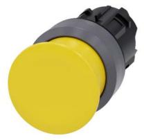
Mushroom pushbutton, 22 mm, round, plastic with metal front ring, yellow, 30 mm, momentary contact type, with laser labeling, symbol number according to, ISO 7000 or IEC 60417
