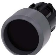
Pushbutton, 22 mm, round, plastic with metal front ring, black, Front ring, raised momentary contact type, with laser labeling, lower case
